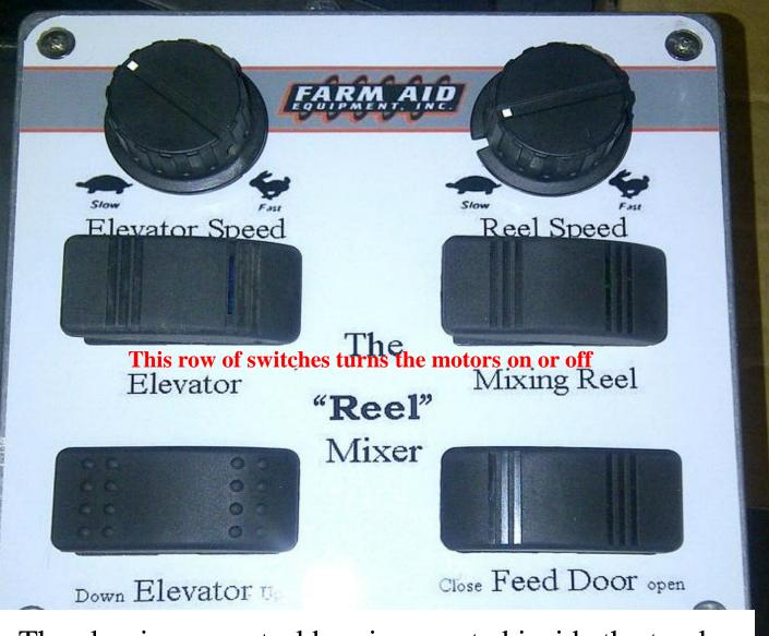
The aluminum control box is mounted inside the truck.
