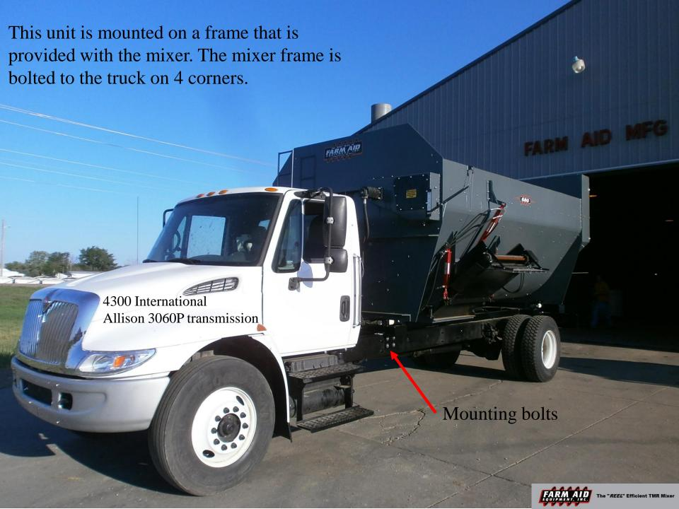
Our frame starts out as a 6" X 6" steel tube, The tube is cut out so that the cut tube straddles the truck frame. Measurements are taken of the frame and 3/8" steel plate is cut to fit the truck frame with a window in it where the 6" X 6" tube passes through. The tube is welded to the tube after the plate is bolted to the truck and the diagonals are checked ensuring accurate operation of the weigh bars
